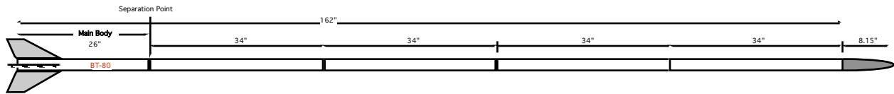
The lower main body was from an old F Superroc Duration model, from around 1982. It was given four BT-80 tube sections (when flown as an F Superroc Duration model, it was only around 8 feet or 250 CM tall). The couplers were 8.5" long, 4.25" inside each tube, for an aspect ratio of 1.66 to 1. The couplers were originally a little bit loose, so tape was added to make them friction fit tightly. The joints were taped with package tape.
