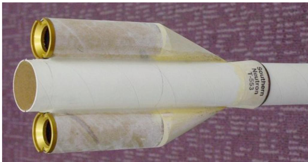
The design was for one F10 and two E6's, somewhat similar to the March model #4, but shorter and with drag reduced. The drag reduction included fairing in the 24mm engine pod noses ("Soyuz booster" style), and changing the fin orientation 45 degrees so two fins would be glued to the pods and two fins at 90 degrees to the pods. Another change was to boat-tail the model by going down from BT-55 to a 30mm tube for the last 10 inches of the tail section.
