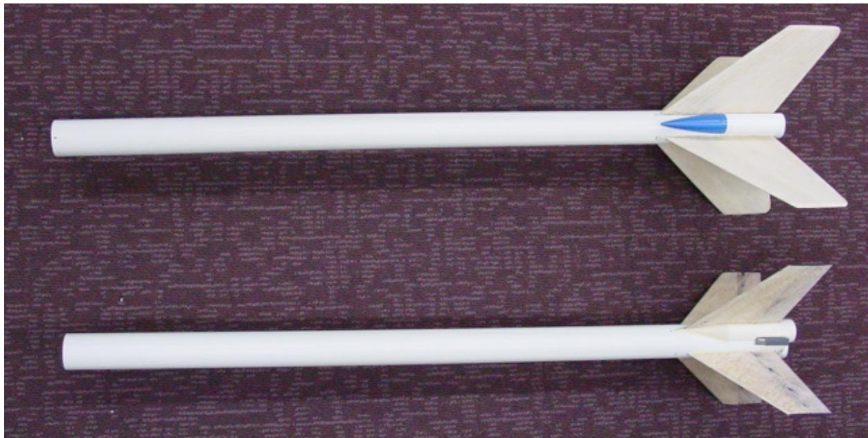
In the above photo, the lowermost main body of Model #4 is at the top (blue noses on 24mm sidepods), and model #7 is at the bottom. The upper sections will be identical, four 34" long BT-60 with 8.5" joiners.
