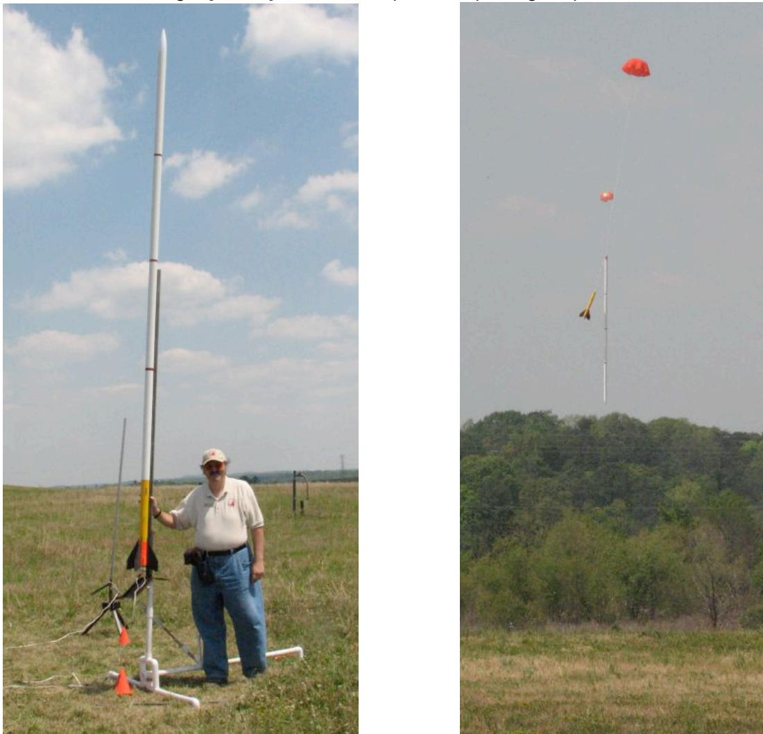
The main body of that model used to fly on four D12's. For this flight, it was flown on four E9's. The propellant mass technically made it an HPR model, in order to have been legal G Superroc it would have needed to fly on two E9's and two D12's. It ignited all four E9's, and
