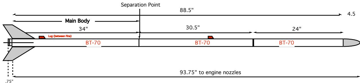
It was all-BT-70, close to minimum length, at 238 CM. Instead of a G40, the engine choice was a cluster of three E9's. This model was intended as a back-up model to Ryan's, and was flown for the second official contest flight. It flew successfully, tracked to 419 meters. That gave it a score of 99,722 points, which won the contest for Team Division and set the record for G Superroc Alt for Teams (no record existed before that).
