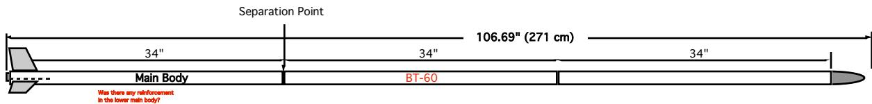
It was based on a similar model that has been successfully test-flown by Launch Crue member Jim Stum. The length was 271 CM, 46 CM over minimum.
