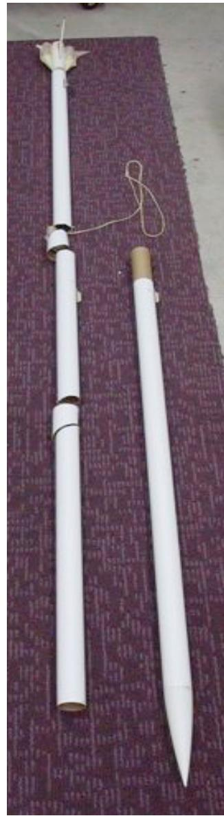
Later Rocksim analysis indicated that this model probably flew 100 ft/sec faster than the max. length BT-60 Model #4 in March. Sims indicated model #6 flying at 399 ft/sec compared to 299 ft/sec for Model #4. That means that Model #6 flew 33.4% faster than Model #4, and had 78% more aerodynamic loads on it than Model #4.
